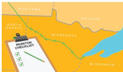
**5. Monitor the Right of Way:** Monitor the Right of Way with regular pipeline patrols, pipeline signs indicating exact location, depth of cover surveys and "Call Before You Dig" Programs.
